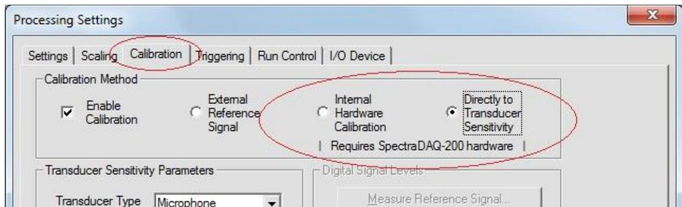
Because the DAQ input voltage is known, direct calibration methods can be used:
