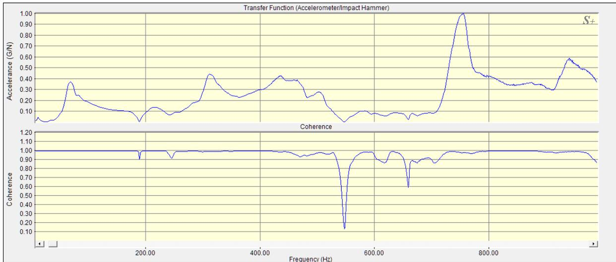
The transfer function these two channels produces a plot of Accelerance (acceleration/force)
